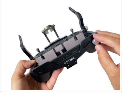
Use the small (M3x6mm) screws and hex key provided to fix the Kraken front plate to the LifThor RC PRO mount as shown.
