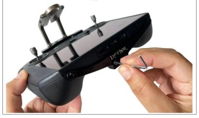
Once the extension arms for the LifThor KRAKEN's plate are fixed (step 1), align the plate with the controllers mounting point and secure it with the (x2) M4 screws.
