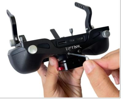
Remove the lower bracket of the quick release mount to fix it to your preferred tripod. Note the quick release bracket is universal so it can be mounted with either of the two mounting holes or both. Either way it will be secure properly.
