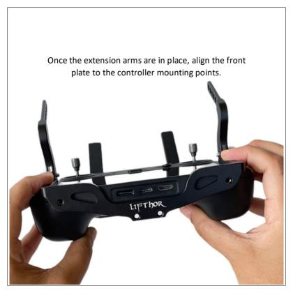
Secure the controller in place with the remaining (2x)M4 thumb screws provided. We recommend to place both screws before tightening them to maintain the alignment.
