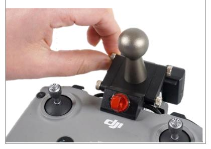
Remove the TRIPLTEK bracket by unscrewing the tripod knob from the mounting bracket.
