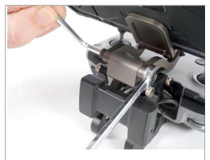
Once you have adjusted the preferred position/height you can tighten the extension arms on the back with the help of an 8mm wrench key to secure it in place.
