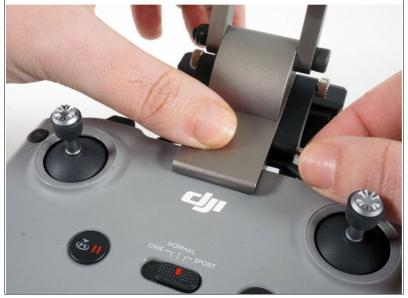
Finish screwing the two rear screws to properly secure the mounting bracket
