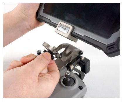
Mount your TRIPLTEK Tablet to your remote control by securing it with the tripod knob provided. Make sure to properly adjust the preferred position.
