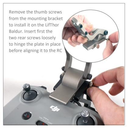
Once everything is in place, pressure the plate against the RC to secure it in place and proceed to screw the remaining two screws. There is no need to force the screw tight
