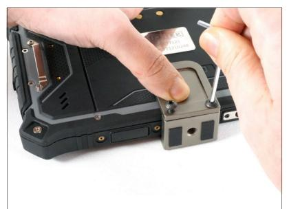
Secure the bracket in place by attaching the rear piece. We recommend placing both screws before securing it tightly, to help it keeping it aligned. Once secured your TRIPLTEK tablet is ready to be mounted.
