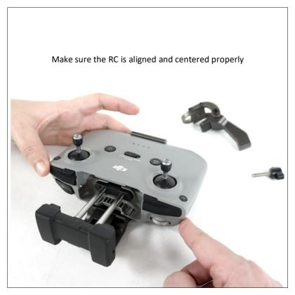
Reconnect the neck of the aluminum base between the antenna bars back to the main body.
