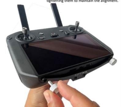
Apply pressure with your thumb to secure the lower frame to install the back of the mount, make sure the mount is properly aligned and has a tight grasp of the controller. It's recommended to extend the
