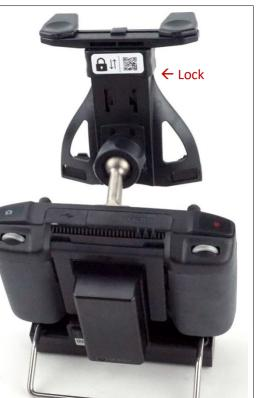
Place the tablet in landscape mode by pulling the spring mechanism upwards and release it to secure the tablet in place. You can adjust the top clamp tabs, if needed, to avoid pressing on any buttons
