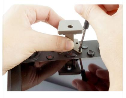
To have better access of the rear screws adjust the angle of the top bracket
