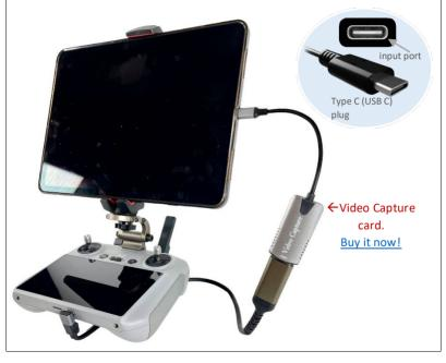
It's <u>only possible</u> to connect those tablets with a Type C (USB C) input port, meaning those tablets that use a Type C Cable to charge. If your tablet uses a Micro USB or Lightning cable you won't be able to connect to your RC2
