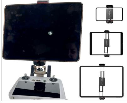
Please note to be able to connect the RC2 with any Tablet (Apple or Android) you will need a Video Capture card – *not included*- and a tablet with Type C (USB C) input port
