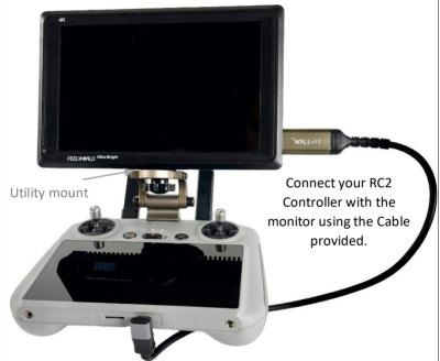
Using the  $(\frac{1}{2}-20)$  knob screw provided, screw the monitor in place through the top opening of the utility mount and secure it tightly.
