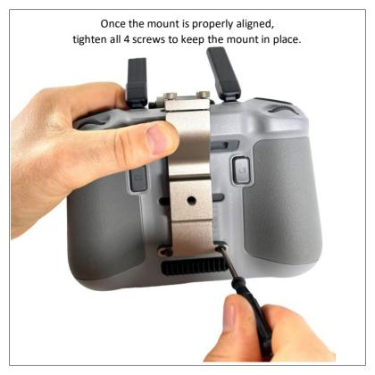
If needed, to adjust the angle of the utility mount you can loosen it up using the hex key and wrench provided.
