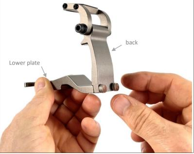
Align the controller with the mount's lower plate to get access to the controller's mounting points. Hold it in place by using the (2x) 2.5x8mm screws, leave it loosely for now. Re-attach the back piece with the (2x) thumb screws - not too tight since you will still need to be able to align properly the mount to the RC. Make sure the mount is properly aligned and positioned between the middle of the antennas. If you are having trouble aligning the mount release more pressure of the screws
