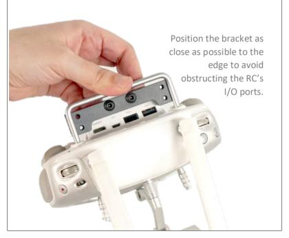
Secure the tripod bracket back with the screws, you can insert all screws before tightening them to have the mount aligned while you secure the bracket
