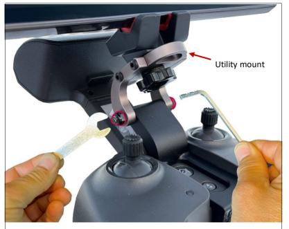
Loosen up the utility mount using the hex key and wrench provided to adjust its angle.
